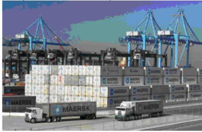
\* Caution: Trucks pulling container trailers should not be counted as port trucks. A container trailer (typically 53' long) is a single unit and can not be separated into a chassis and container. The container is built on the chassis. Furthermore, the container will NOT have the vertical ribbing seen with port container trucks. These trucks are NOT PORT TRUCKS and should NOT BE COUNTED.
