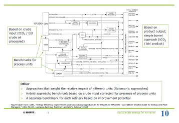
Solomon's benchmarking methodologies allow comparing refineries with different sizes and configurations
