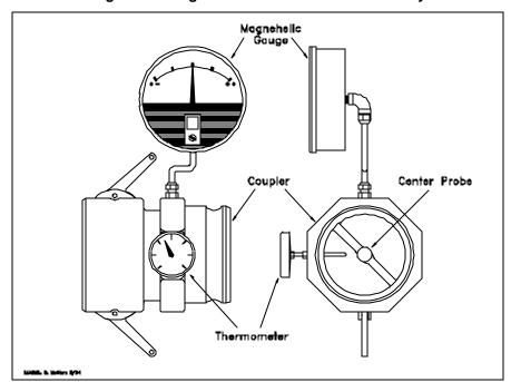
Figure 1 - Cargo Tank Back Pressure Assembly
