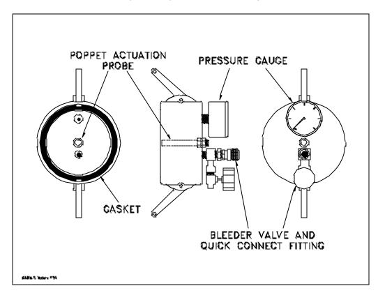
Figure 2 Vapor Coupler Test Assembly
