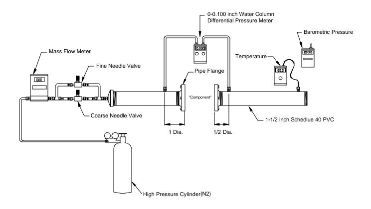
Notes: Three tube configurations are required to measure different components. Each configuration requires a uniquely designed orifice plate, flange, couplings, and male & female interfacing adapters.
