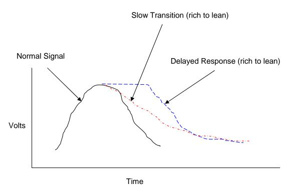
Fig. 1: O2 Sensor Deterioration Sketch
