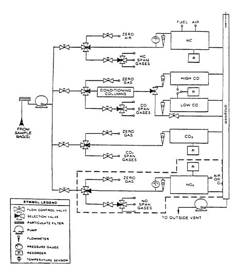
FIGURE F90-3: Exhaust Gas Analytical System
