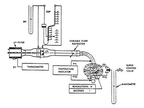
FIGURE F78-5:-PDP-CVS Calibration Configuration.
