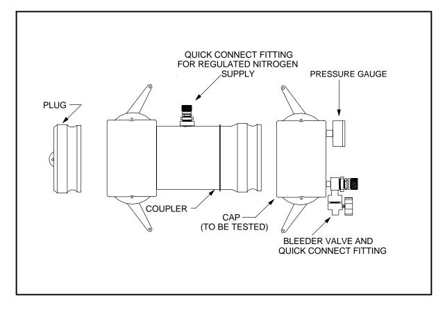
Figure 3 Vapor Coupler Test Assembly
