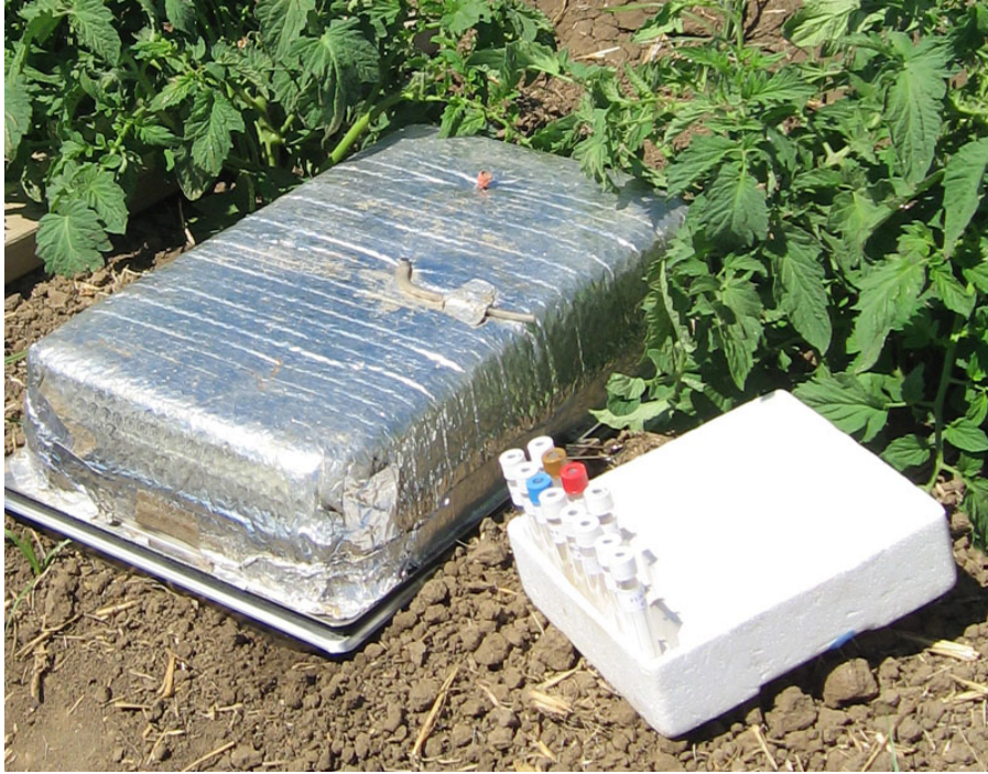
Figure 1A. Vented chamber used for nitrous oxide flux measurements in the field and exetainers used to store the air samples.
