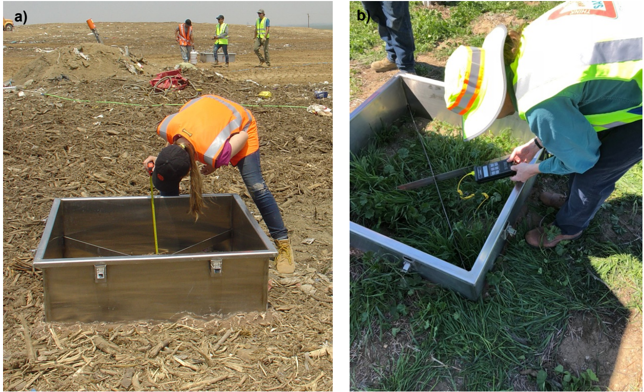
Figure 3.12 Post-Flux Tests Prior to Removal of Chamber Collar
